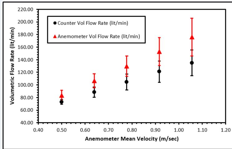
Figure 7: volume flow rate measured by gas meter and anemometer for different anemometer velocities
