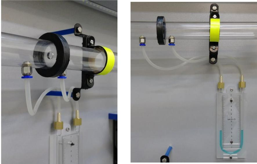
Figure 6: Orifice plate for measuring static pressure
