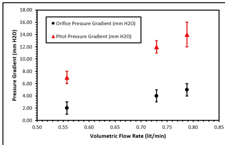
Figure 9: pressure gradient orifice plate and Pitot tube for different volume flow rate
