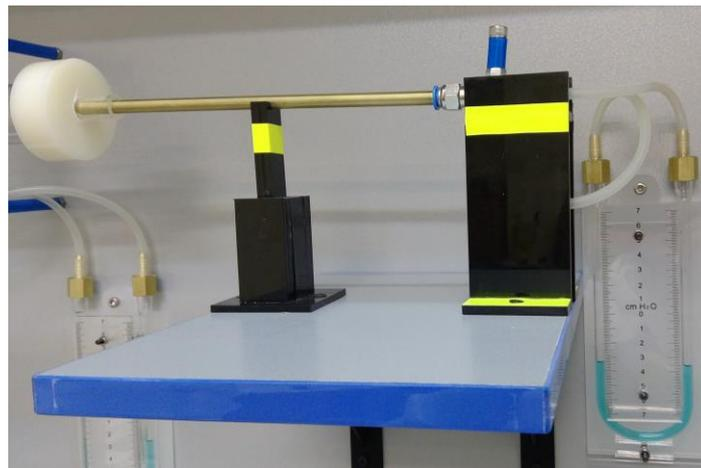
Figure 5: Pitot tube is used in apparatus
