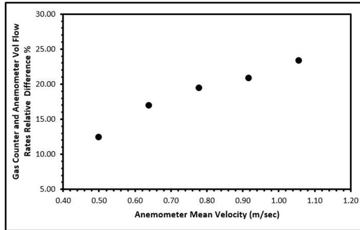
Figure 8: Volumetric flow rate relative error between gas meter and anemometer
