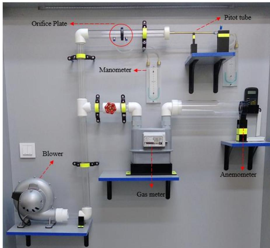
Figure 1: Gases velocity and flow measurement apparatus
