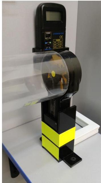
Figure 3: Anemometer for measuring air velocity
