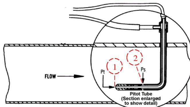
Figure 4: schematic Pitot tube [8]
