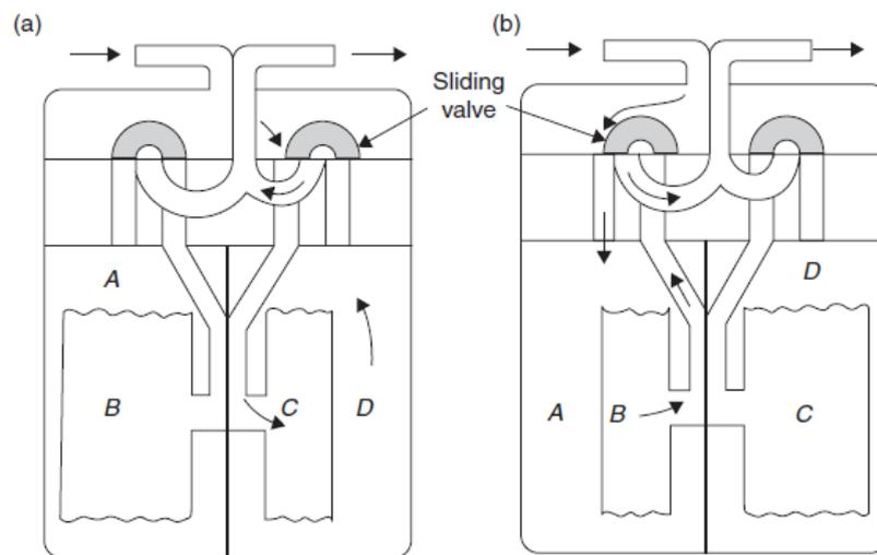
Figure 2: Diaphragm meter. (a) A, empty; B, full; C, filling; D, emptying; (b) A, filling; B, emptying; C, full; D, empty [10]
