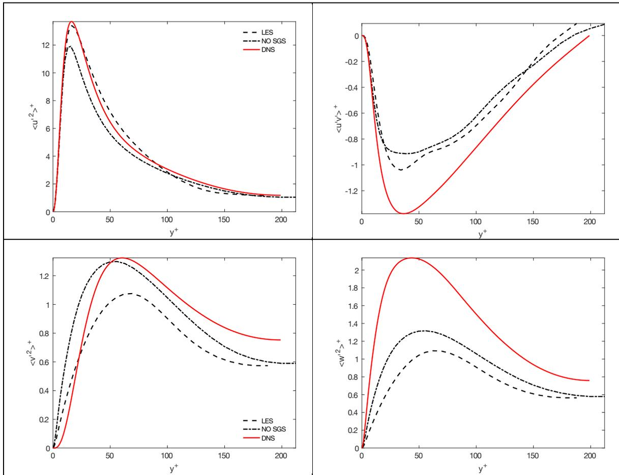
Figure 3: Mean Reynolds stresses in wall units.
