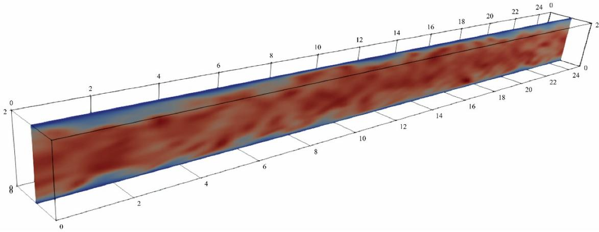
Figure 1: Schematic of the duct flow simulation set-up with a contour plot of the instantaneous streamwise velocity.
