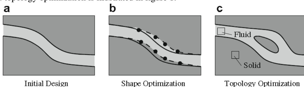
Figure 1: Comparison of shape and topology optimization
