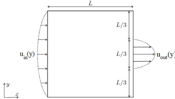
Figure 2: Diffuser design domain with inlet and outlet conditions
