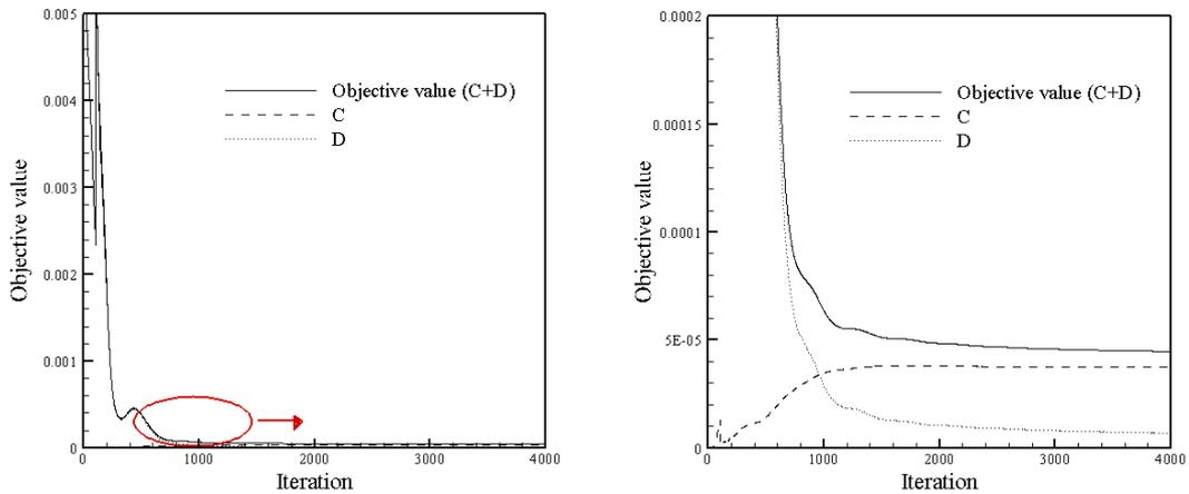
Figure 4: Convergence pattern of the objective function for the diffuser
