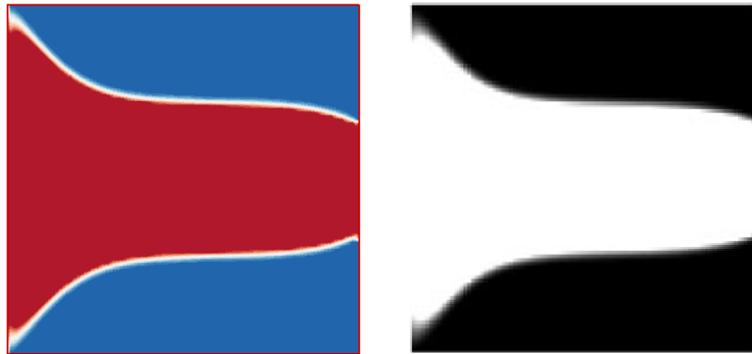
Figure 3: Optimal design for a diffuser at  $Re=10$  on a  $100 \times 100$  lattice (left) in this paper (right) in [6]
