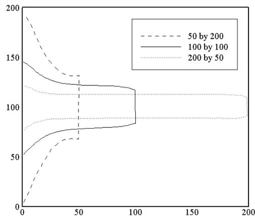
Figure 5: Optimum Diffuser with different domain aspect ratios and constant  $\bar{V}$
